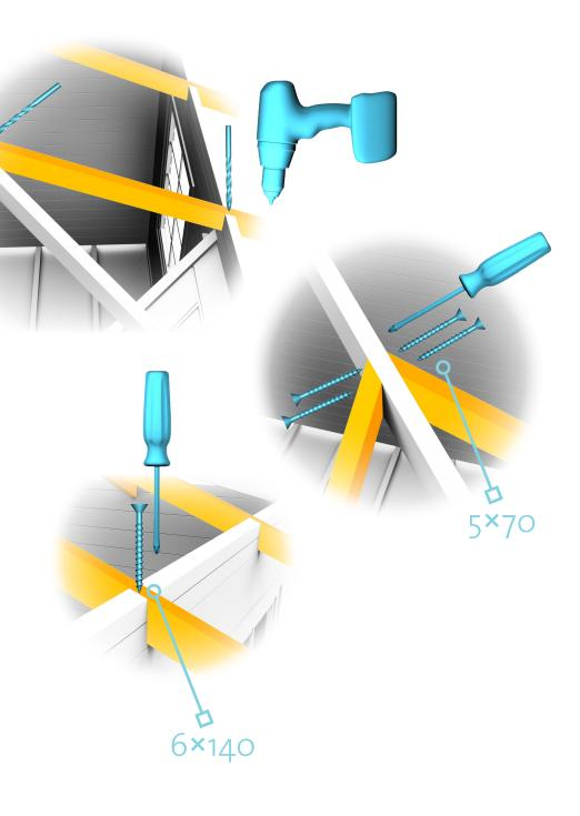
PLACE THE FIRST ROOFBOARD FLUSH WITH THE END OF THE PURLINS AND ATTACH WITH SCREWS
