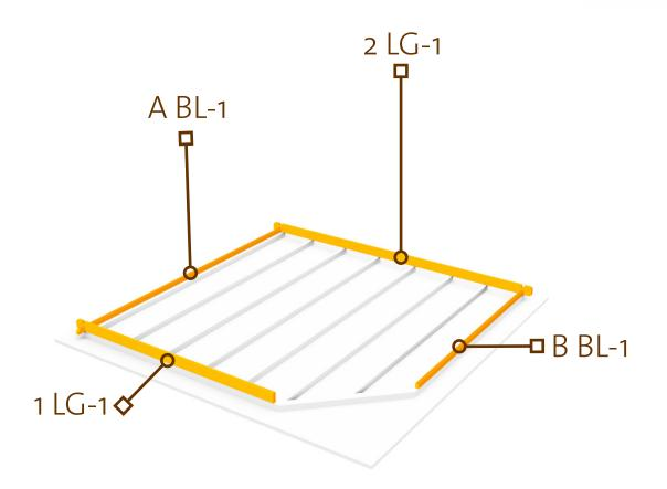
**ATTACH** LOGS TO THE FOUNDATION. × 6 <sup>071</sup>× 12 5×70 Ø4mm Ø 5 mm 5mm 6×140 5×70
