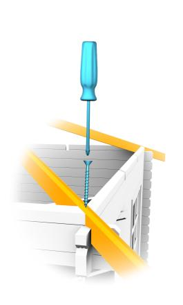
INSTALL THE **ROOF** PURLINS (RFB) AND ATTACH THEM WITH SCREWS.
